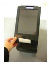
Close the lid, making sure the lid locks into place with the paper coming out. The printer automatically feeds and cuts the paper.
