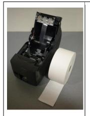
Lift up on the release lever located on the right corner of the printer to pop open the interior lid.
