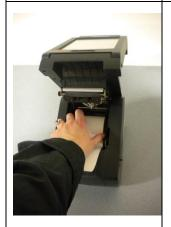
Place a new roll into the housing area, making sure the paper feeds from the bottom of the roll.
