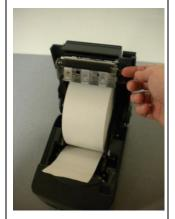
Place a new roll into the paper housing area, making sure the leading edge of the paper feeds from the bottom of the roll.
